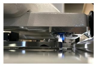
Both screws can be adjusted with the quilting machine on the carriage. Pull the machine to the front to access the front screw and to the rear to access the rear screw.
