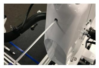
2. Install the black box power cable (see parts list, item N) into the front face cover circuit board to power the black box on the tablet mount.
