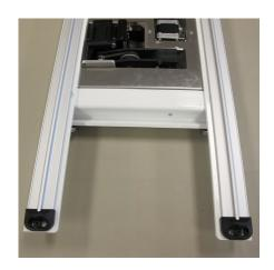
2. Place the Pro-Stitcher carriage on the frame. Starting at one end of the table, begin mounting the blue Flexirack to the front of the table while aligning it to the front white gear on the carriage.
