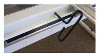
10. With the power cable plugged in and the motors in the engaged position (use the manual engagement/disengagement tool if necessary), ensure that as the quilting machine is moved in both the X and the Y directions, the corresponding gears are rotating, as well.
