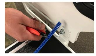
6. At both ends of the blue Flexirack, use two of the small metal clamps (see Parts List, item C) to hold the ends firmly in place. The clamps have a hole through the center and a lip on one end. The lip should be on the side opposite the blue Flexirack. Place the clamps where they will be attached and drill pilot holes using the 3/32-inch drill bit and then use a Phillips screwdriver to fasten the clamps on both sides of the Flexirack to the table.
