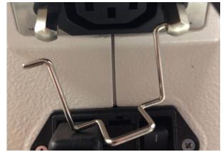
7. Plug the short power cord (see Parts List, item I-2) into the connection panel and into the Pro-Stitcher carriage, securing both ends by pressing the wire cord-retainer onto the cord.
