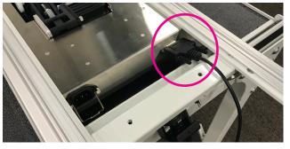
6. Place the ends of the power cord-retaining clamp (see Parts List, item T) into the holes on the retainer screws on the back connection panel. The u-shape should be aiming down so it can go down over the plug to retain the cord inside the machine connector.
