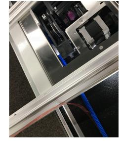
3. Use the carriage as a guide and align the blue Flexirack with the white gear along the length of the table (see arrow at right), removing the pink protective layer and pressing downward on the blue Flexirack while moving the carriage down the entire length of the table.
