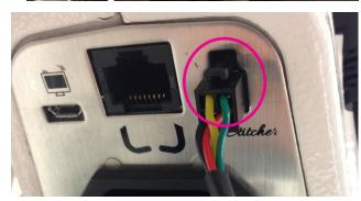
5. Plug the large end of the Pro-Stitcher carriage communication cable (see Parts List, item M) into the back of the carriage (right side as seen from back of machine). Tighten the black screws using a flat-head screwdriver.
