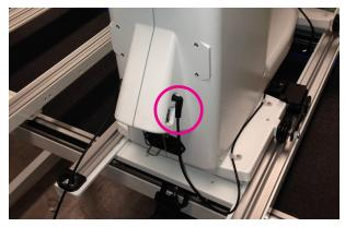
3. Plug the end of the carriage encoder cable (X) into the round connector above the square laser connection as shown.
