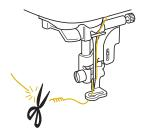
• If the thread is left at the beginning of the stitching, it may be embroidered over as you continue embroidering the pattern, making it very difficult to remove the excess thread after the pattern is finished. Trim the thread at the beginning.
