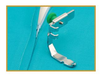
4. Turn the handwheel toward you to lower the needle. Adjust the position of the foot relative to the needle using the adjustment screw to slide the foot from left to right. Then tighten the zipper foot adjustment screw.
