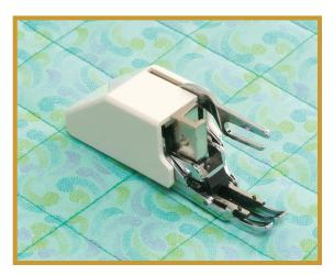
4. Tighten the screw securely with the screwdriver. Tightening adequately is important as the screw might loosen due to the foot and forked operation lever vibration.
