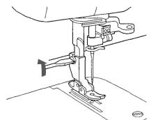
3. Insert the forked part of the operation lever while raised in an upright position onto the screw on the right side of the needle bar, as shown and then insert the capscrew.
