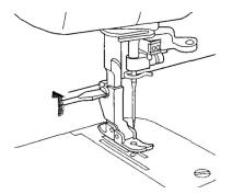
3. Attach the 8mm Bi-level Spring Action Guide foot and tighten the screw.
