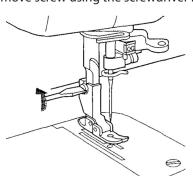
3. Attach the 5mm Bi-level Spring Action Guide foot and tighten the screw.
