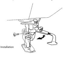
2. To adjust, lightly loosen both screws to move the guide left, right, forward or back. (See arrows in illustration). Remember to tighten the screws before stitching.
